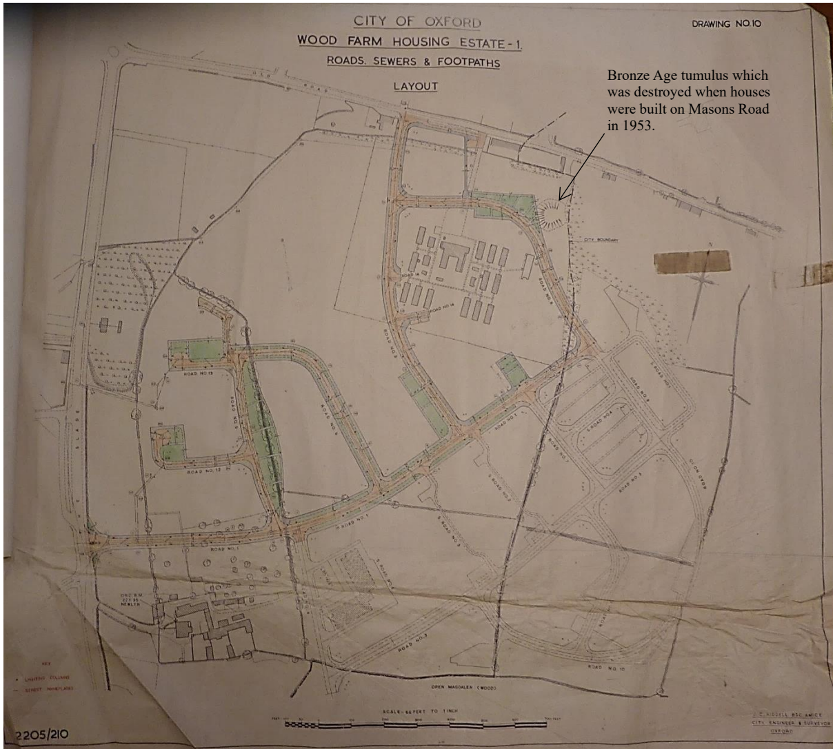
Plan of the Wood Farm Estate, 1951, by the City Engineer and Surveyor JC Riddell, showing proposed roads (numbered but not yet named), sewers and footpaths, overlaid with the existing field boundaries. The Old Road Camp can be seen upper centre, and the buildings of Wood Farm itself are lower left. Sections 1 and 2 of the estate, north of Wood Farm Road, are shown coloured on this plan; section 3, south of Wood Farm Road, is shown in black and white. Notice that the city boundary ran through the estate. Image courtesy of Oxfordshire County Council, Oxfordshire History Centre, OCA 3/2/Y3/26/1.
